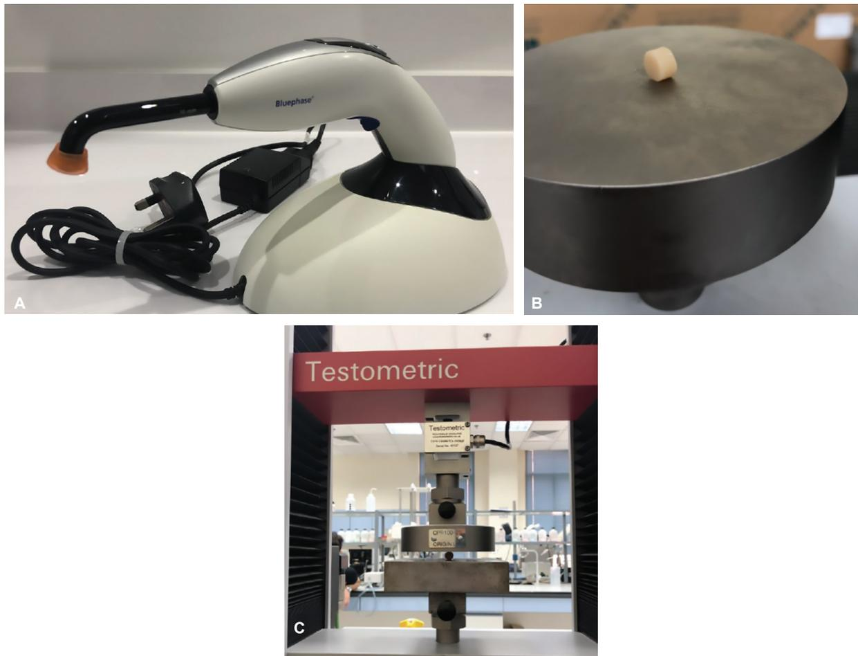
**Figs 1A to C:** Devices and composite specimen used in this study. (A) Blue phase G2 light curing unit; (B) Cylindrical composite specimen of 6 mm in diameter and 4 mm in height; (C) The universal testing machine (Testometric/UK)
