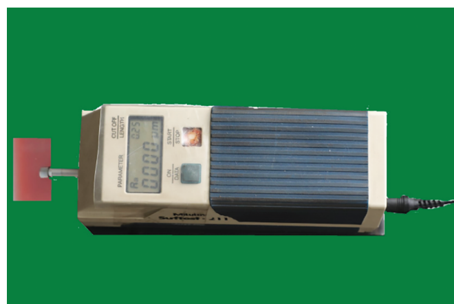
Fig. 1: Profilometer being used to analyze the surface roughness ( R_a ) (screen showing the digital measurement of surface roughness of the specimen being displayed)
