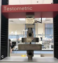
Figs 1A to C: Devices and composite specimen used in this study. (A) Blue phase G2 light curing unit; (B) Cylindrical composite specimen of 6 mm in diameter and 4 mm in height; (C) The universal testing machine (Testometric/UK)
