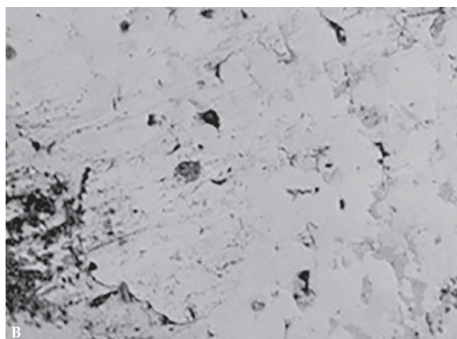
Figs 15A and B: The SEM investigation of the stainless steel bracket during fretting in artificial saliva pH = 3
