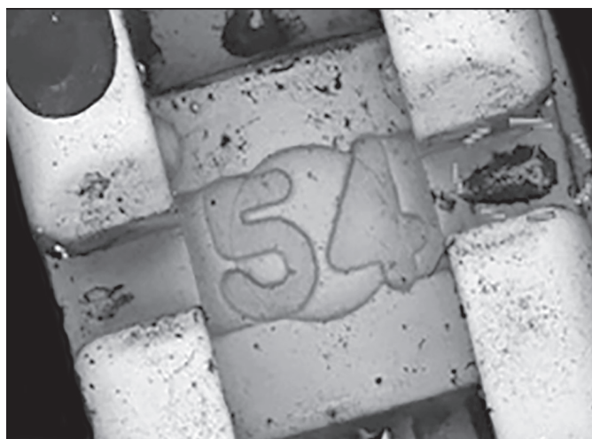
Figs 7A and B: Fretting contact zone on the stainless steel bracket Ti-Ni wire
