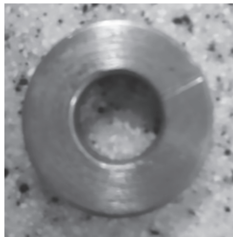
Fig. 1: The metal mold of 6 mm in diameter and 4 mm in thickness used with bulk-fill composites in this study with a small groove indicating the top surface
