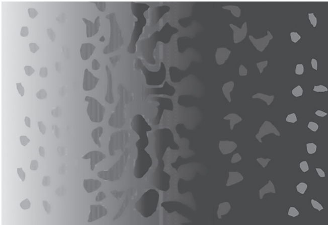
Fig. 1: Schematic representation of a continuously graded microstructure
