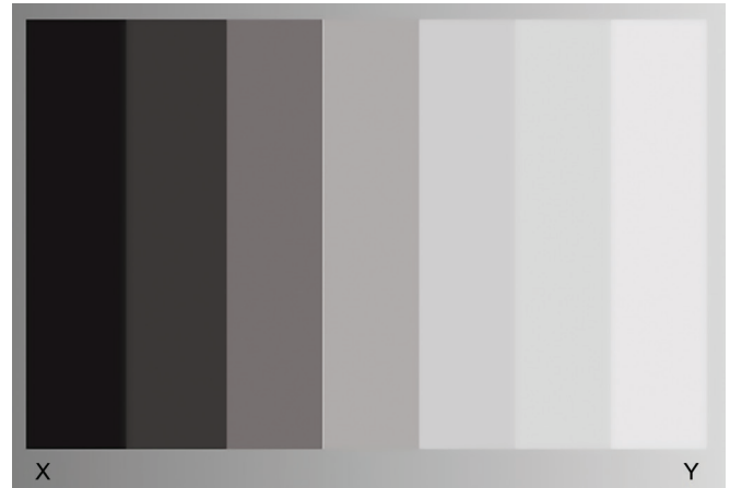
Fig. 2: Schematic representation of a stepwise graded microstructure
