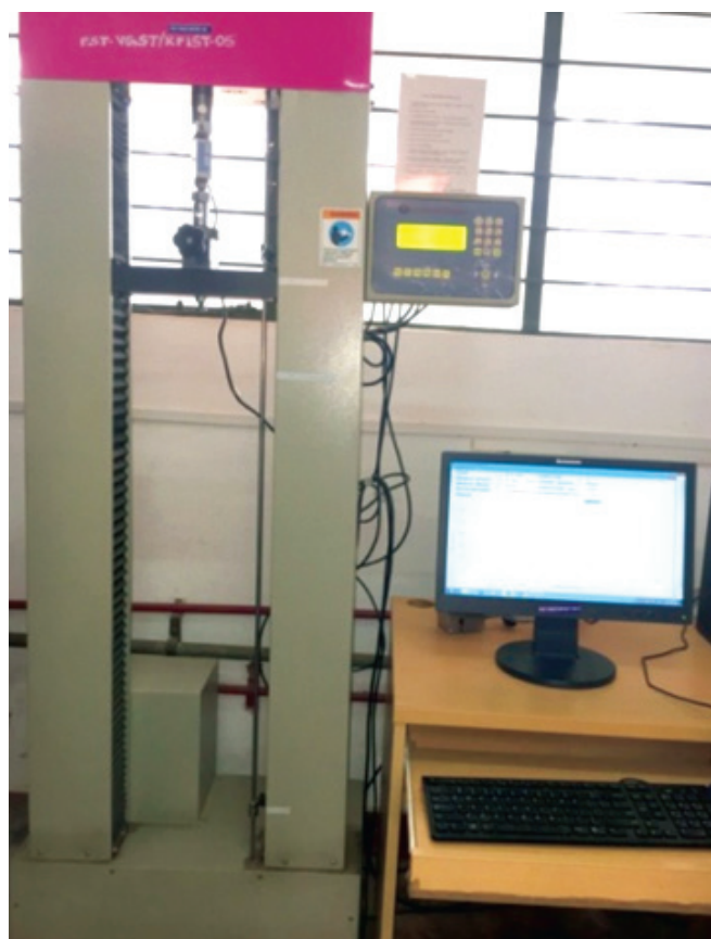
Fig. 5: Hounsfield universal testing machine with appropriate software to record all parameters
