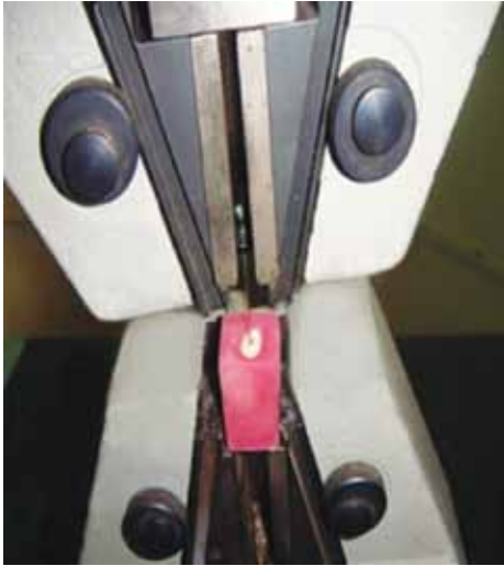
Fig. 1: Finger spreader inserted into the obturated root canal using universal testing machine
