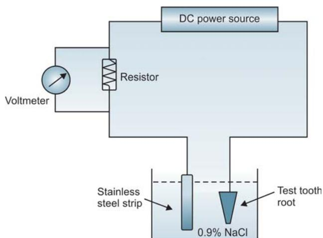
**Fig. 1:** Schematic representation of electrochemical leakage test circuit
