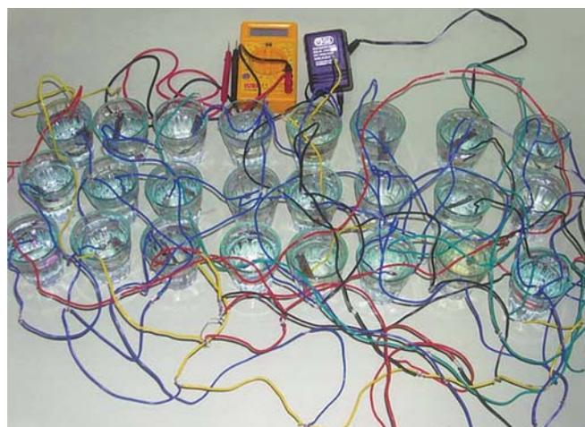
**Fig. 3:** Electrochemical leakage test circuit
