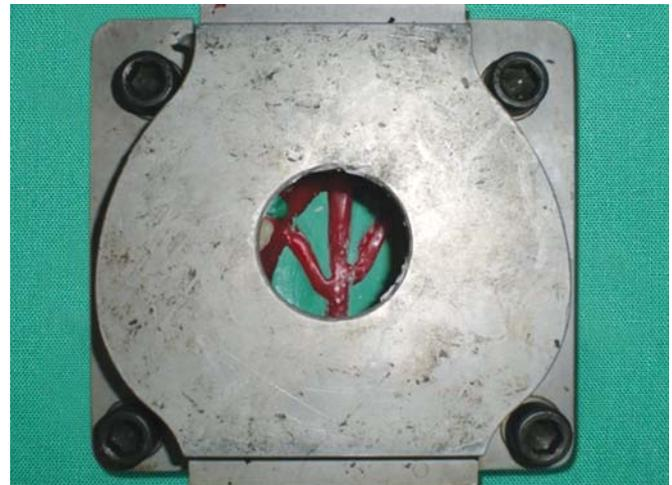
Fig. 3: Injection molding flask
