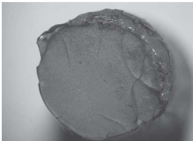
Fig. 1: Example of mixed fracture
