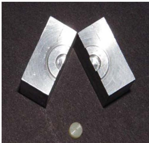
Fig. 7: Retrieval of one sample after splitting the mold
