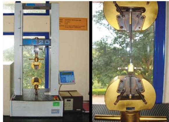
**Fig. 7:** Universal testing machine
