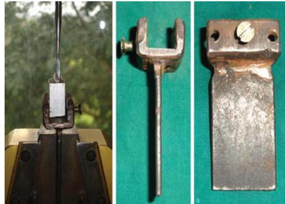
**Fig. 8:** Jig for mounting the specimen to the clamp of the universal testing machine
