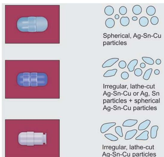
Fig. 3: Amalgam alloys and their structure
