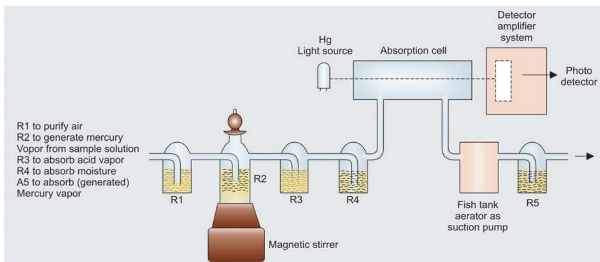
Fig. 1: The vapor generating system with the reaction vessel, four traps and magnetic stirrer is compactly mounted on a sturdy wooden stand with laminated finish
