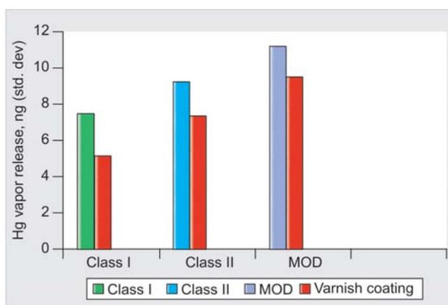
Fig. 7: Cavity design with and without varnish coating
