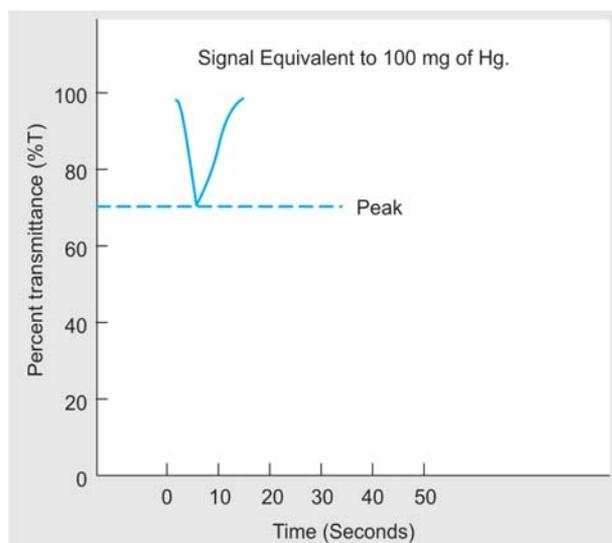
Fig. 2: A plot of the transient signal on the meter as the mercury vapor passes through the absorption cell
